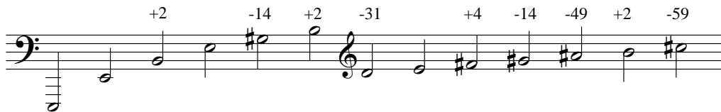
Figure 28: The first 13 partials of E_1 and their deviations from twelve-tone equal temperament, measured in cents.
